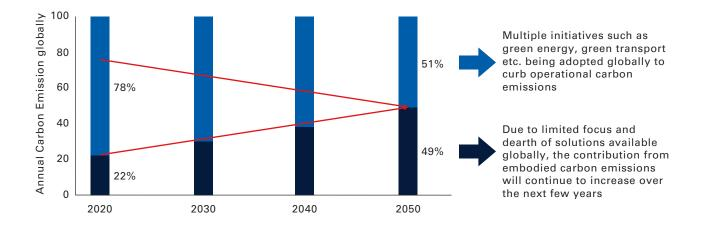
Embodied carbon is conventionally more challenging to track and measure than operational carbon. The latter can be monitored by accessing the energy bills of consumers and manufacturers. Assessing embodied carbon from the finished product alone becomes an arduous task. For project development, it needs self assessment and process transparency across the material manufacturing process and its supply chain.
